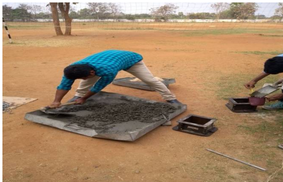
Fig. 1: Hand mixing of concrete
