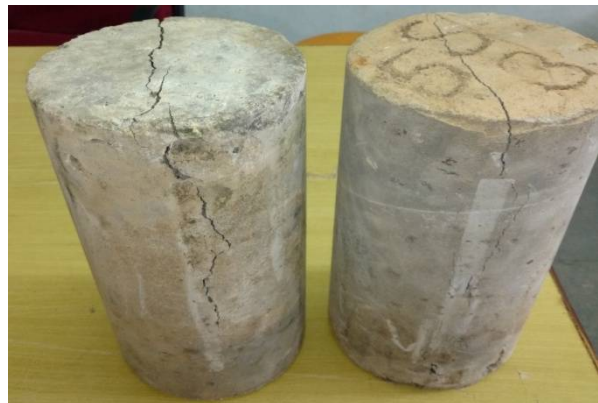
Fig. 6: Cracks pattern observed in cylinders
