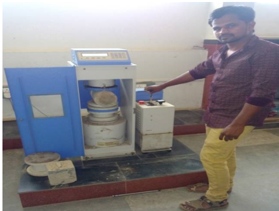
Fig. 5: Cylinder testing setup in CTM
