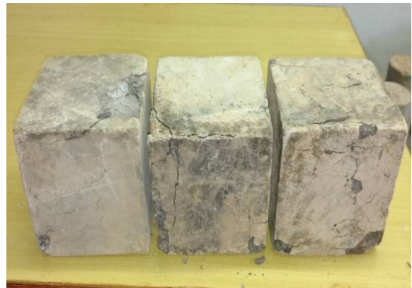
Fig. 4: Cracks pattern observed in cube specimen
