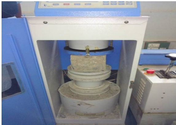
Fig. 3: Compression testing setup in CTM
