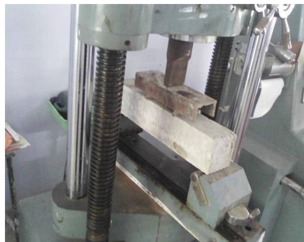
Fig. 8: Flexure strength setup in UTM
